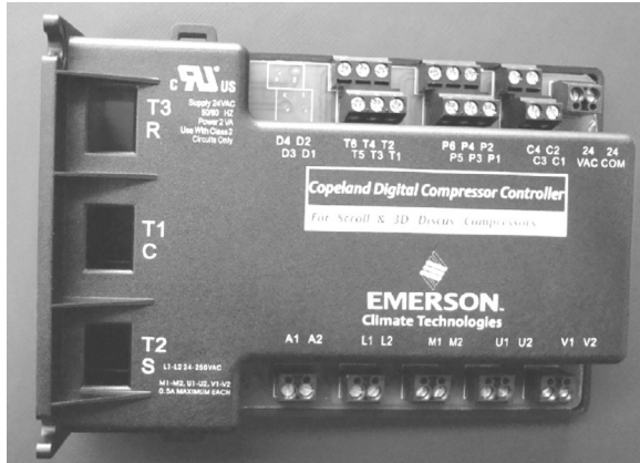
Figure 39 - Variable Capacity Compressor Controller
