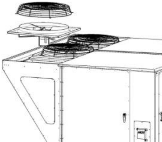
Figure 42 - Removal of a Condenser Fan Assembly
