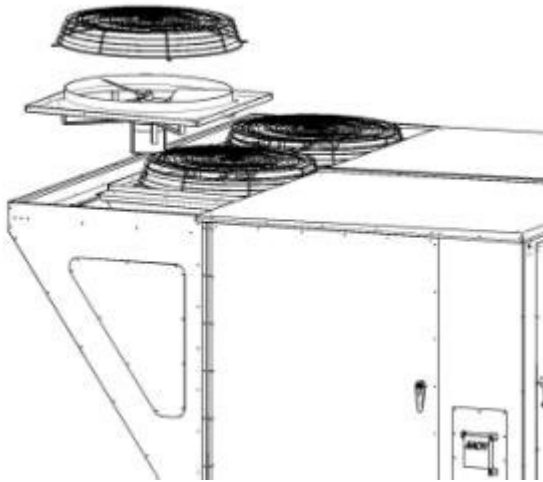
Figure 12 - Removal of a Condenser Fan Assembly
