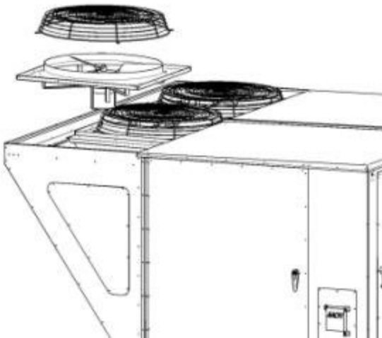
Figure 44 - Removal of a Condenser Fan Assembly
