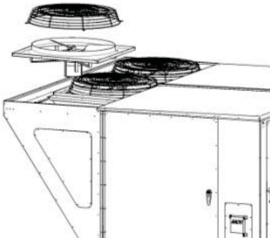
Figure 34 - Removal of a Condenser Fan Assembly
