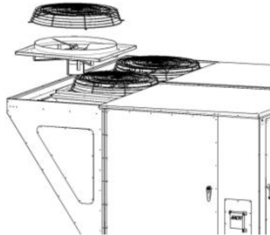
Figure 12 - Removal of a Condenser Fan Assembly
