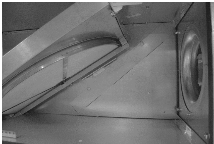
Figure 32 - H3 A or B Cabinet Outside Air Filter Access H3 size A & B outside air filters - access through removing the sheet metal piece shown above.
