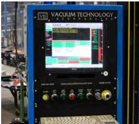
Test interface for the leak test chamber. Operators are able to see real time results.
