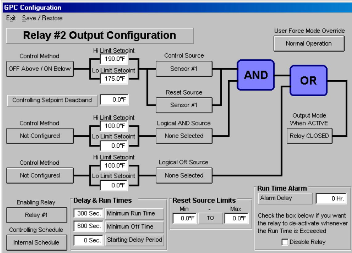
Figure 6 – Relay #2 Output Configuration
