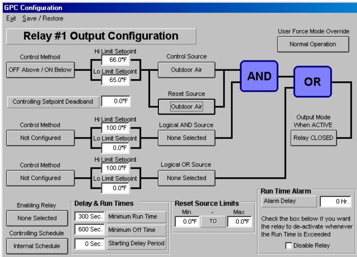
Figure 5 – Relay #1 Output Configuration
