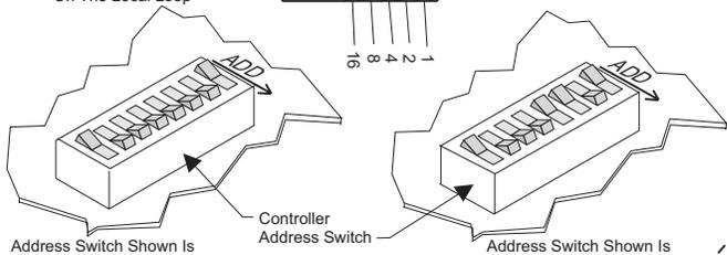
**Caution!** Controller Must Have Address Switch Set Between 1 and 60
