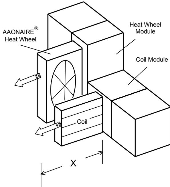
'X' is the minimum required service clearance for heat wheel and coil modules
