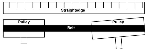
Corrected by moving the position of the motor.
