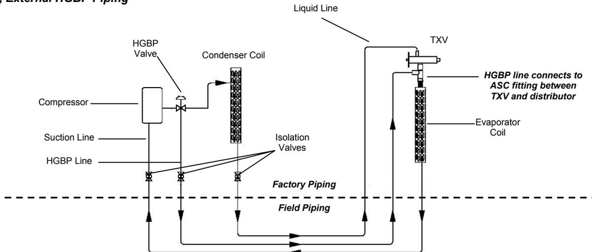
Figure 8.3, HGBP Connection to Evaporator & ASC Fitting
