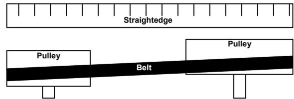
Corrected by adjusting sheaves on one, or both shafts.
