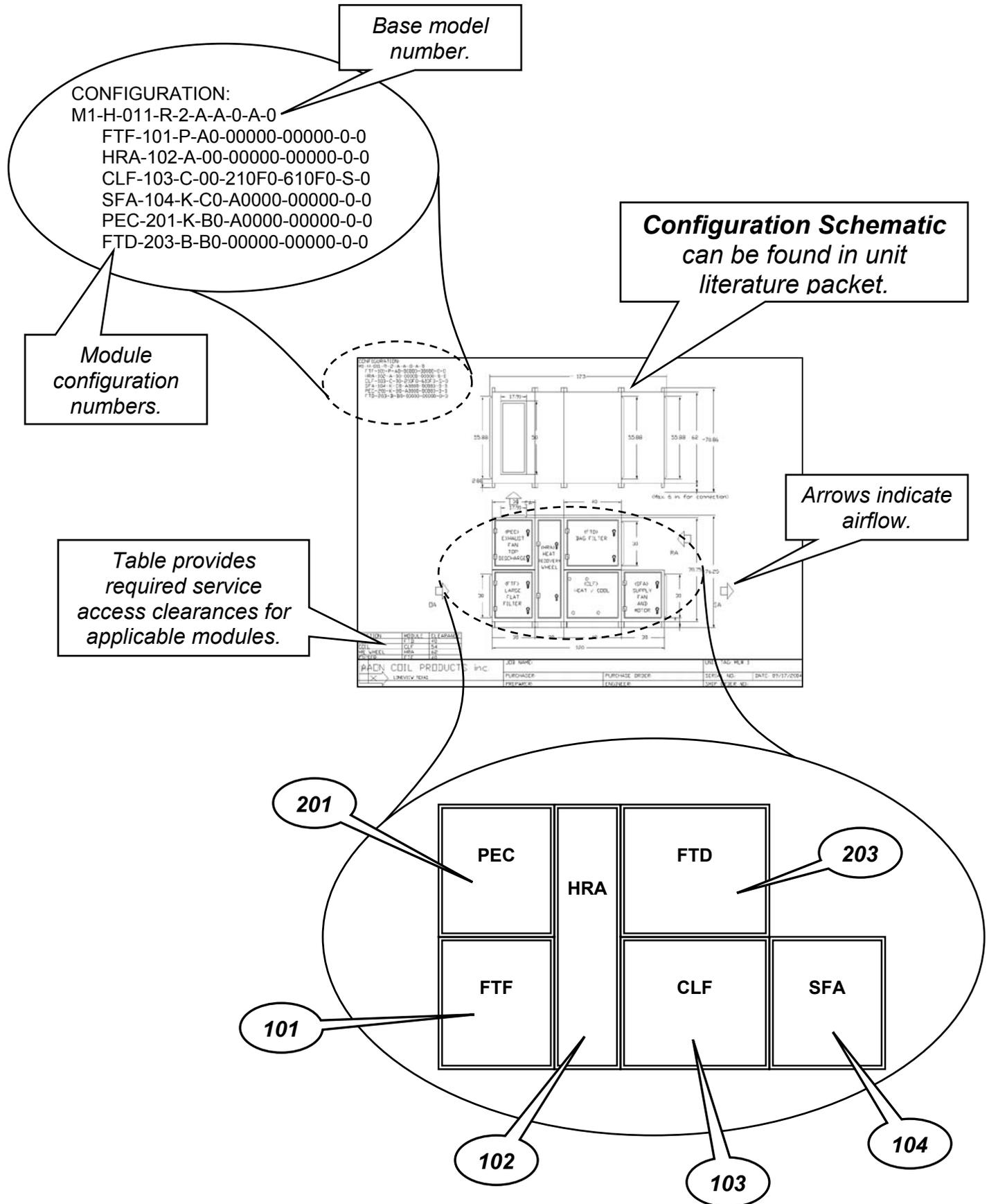
Note that a heat wheel module will have a 100 series number identifying it, but will span both tiers also utilizing a 200 series space, and effectively “skipping” one of the top-tiered numbers.
