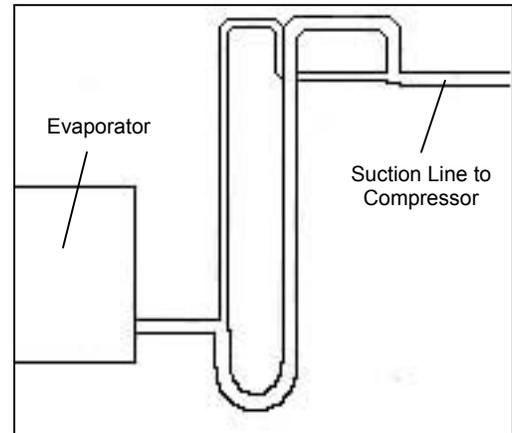
All vertical suction risers should be checked to confirm that oil will be returned to the compressor. Use the tables in this section for pipe sizing information.
