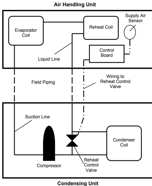
After the room temperature thermostat is satisfied and the humidistat continues to call for moisture removal, the modulating valve will allow a controlled amount of hot gas to enter the reheat coil. A discharge air temperature sensor mounted within the air handling unit provides input to an electronic control board. The valve position is controlled to provide a specific supply air temperature set point that is set on the control board, or sent to the control board by a remote 0 to 10 VDC signal.
