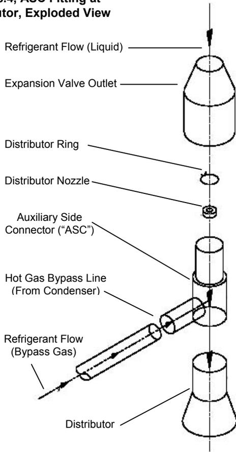
The ASC fitting will come installed by the factory. Should you need to re-install the ASC fitting in the field, then do so according to the following procedure:
