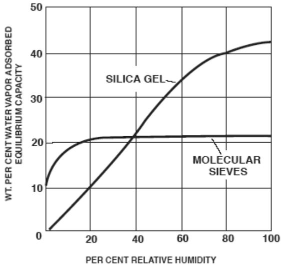
Fig. 1. Effect of relative humidity on desiccant capacity
