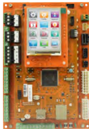
Pioneer Gold with Touchscreen Interface and BACnet IP/MSTP and Modbus
